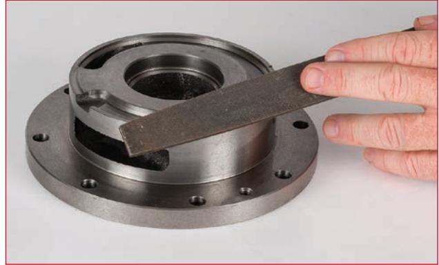
11. Install the pump cover using four bolts. If the impeller still does not lock up after filing the inner edge of the pump cover and removing all shims, it is no longer in tolerance and should be replaced. After installing the new impeller, repeat the shimming process starting with step five.
