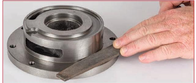
5. Using only one of the two original shims, install the red shim (0.002") with the pump cover using only 4 bolts (alternating holes) and tighten.
