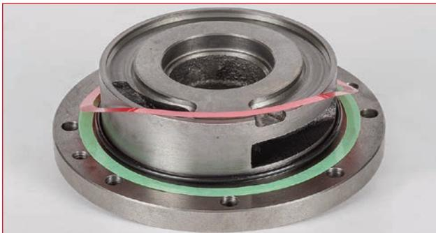
3. Clean the mating surface on the front of the pump case using a file or sandpaper as shown.
