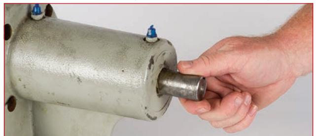
7. If the fan/shaft rotates freely, remove the red shim and install the pump cover using four bolts. Note again whether the impeller rubs or is locked up.
